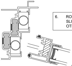
6. ROTATE SASH A LITTLE, SLIDE SASH TO THE SIDE TO CLEAR OFF OTHER PIVOT BAR
